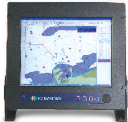
20.1" TFT monitor (larger displays also available) with excellent brightness and contrast levels and direct dimming control. Certified to IEC60945, IEC61174 and IACS E10. Can be panel-mounted or supplied with protective aluminium casing and brackets for desktop, deck-head or wall mounting. Measures 534 x 481 x 223.5mm. Weight 18 Kg.
